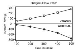
† In vitro tests performed using 3:1 glycerine/saline at 37°C.
